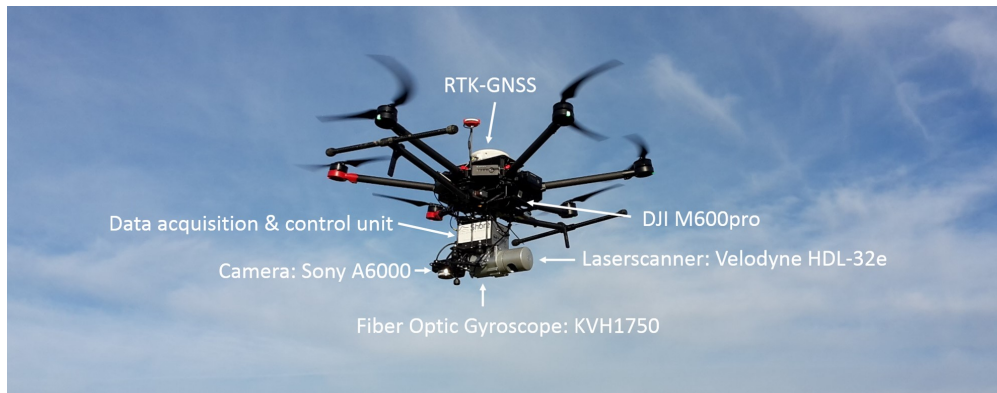
Figure 4.1: Mobile LiDAR system on DJI M600pro. Components annotated.
