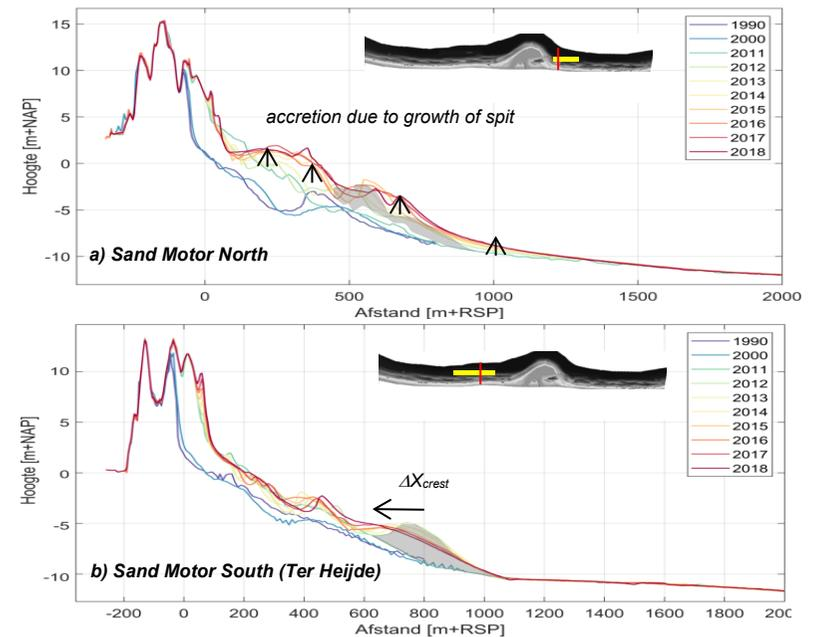
Figure 3.15 Measured cross-shore profiles at the shoreface nourishments close to the Sand Motor. Grey areas demarcate the nourishments (Huisman et al., 2021).
