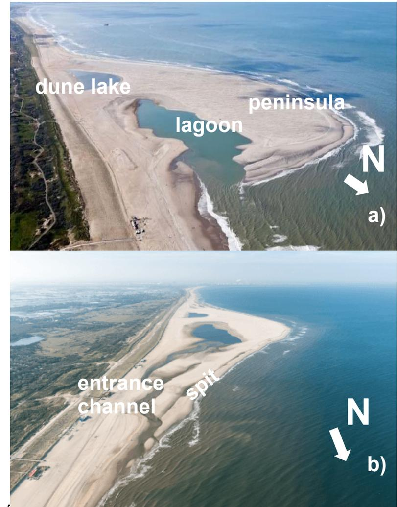
Figure 3.2 The Sand Motor during low tide on a moment shortly after construction in 2011 (a) and in October 2013 (b)
