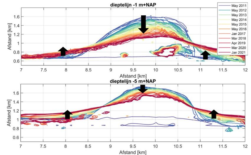
Figure 3.4 Coastline changes at the 1 and 5 meter depth contour of the Sand Motor (Huisman et al., 2021).
