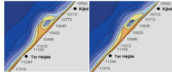
Figure 3.1 The a-priori predicted morphological development of the Sand Motor as computed for the EIA. Left: the computed development after 5 years. Right : the computed morphological change after 10 years.
