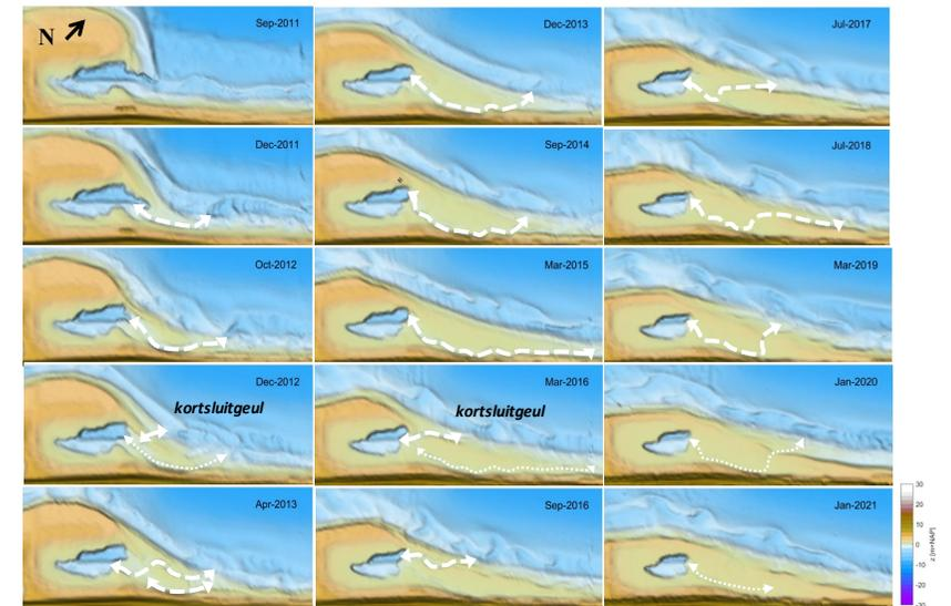
Figure 3.8 Development of the entrance channel at the northern flank of the Sand Motor in the last 10 years. Contour lines show the high-water mark (Huisman et al., 2021).
