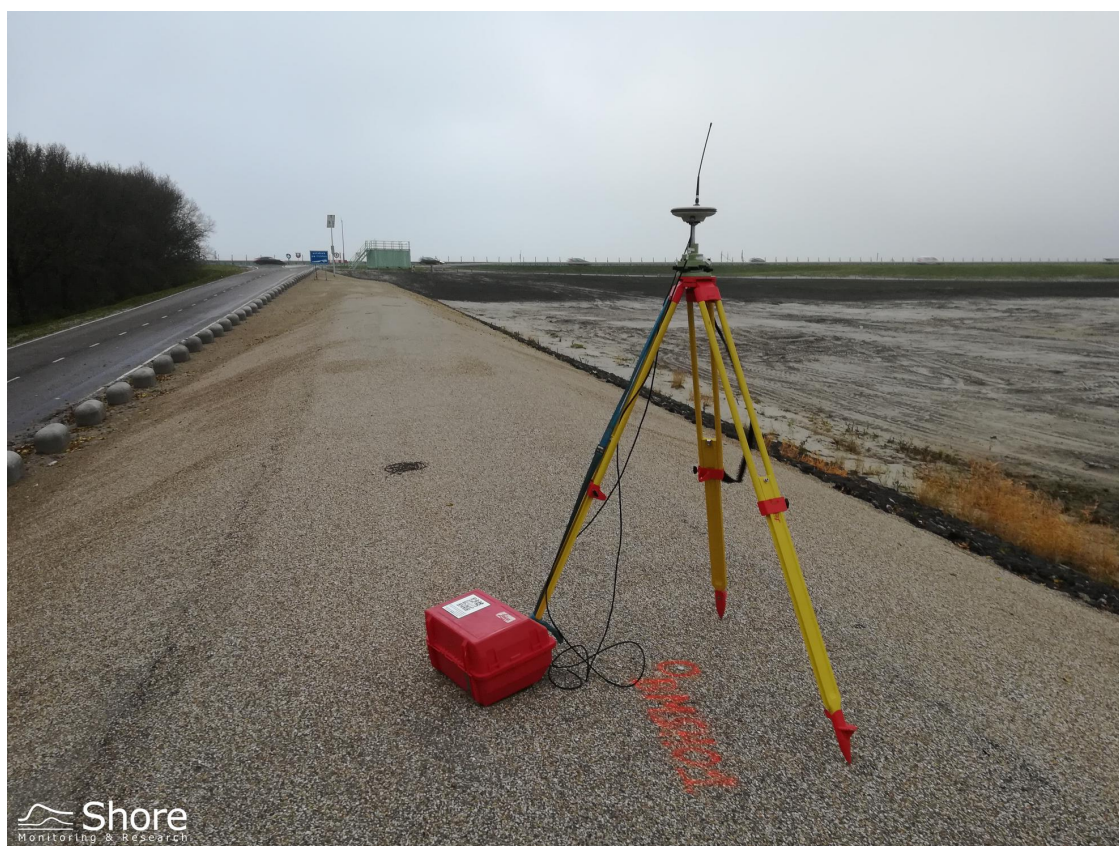
Figure 3.1: GNSS Base station boven BMSH01.
