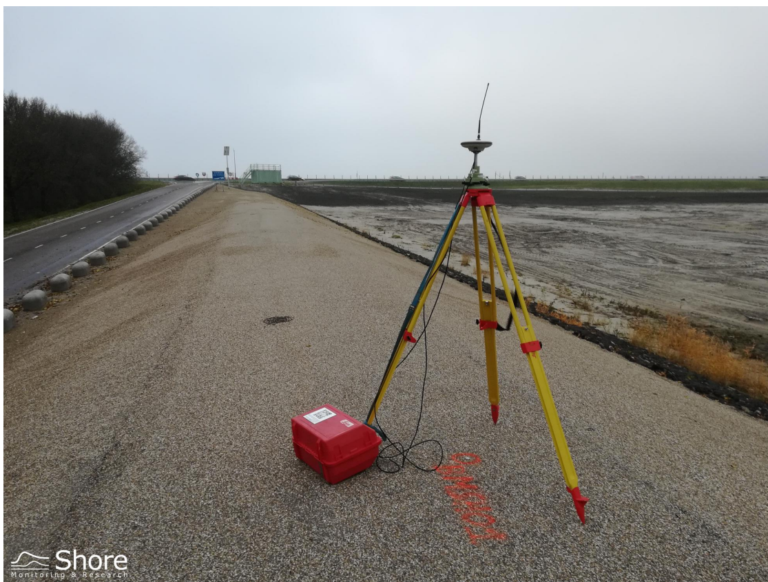
Figure 3.1: GNSS Base station boven BMSH01.
