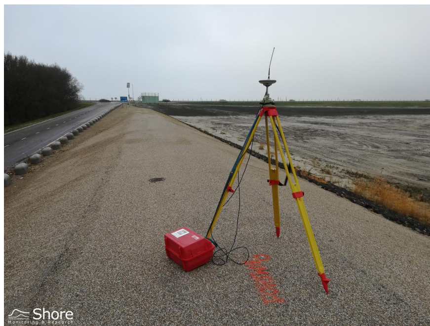
Figure 3.1: GNSS Base station boven BMSH01.
