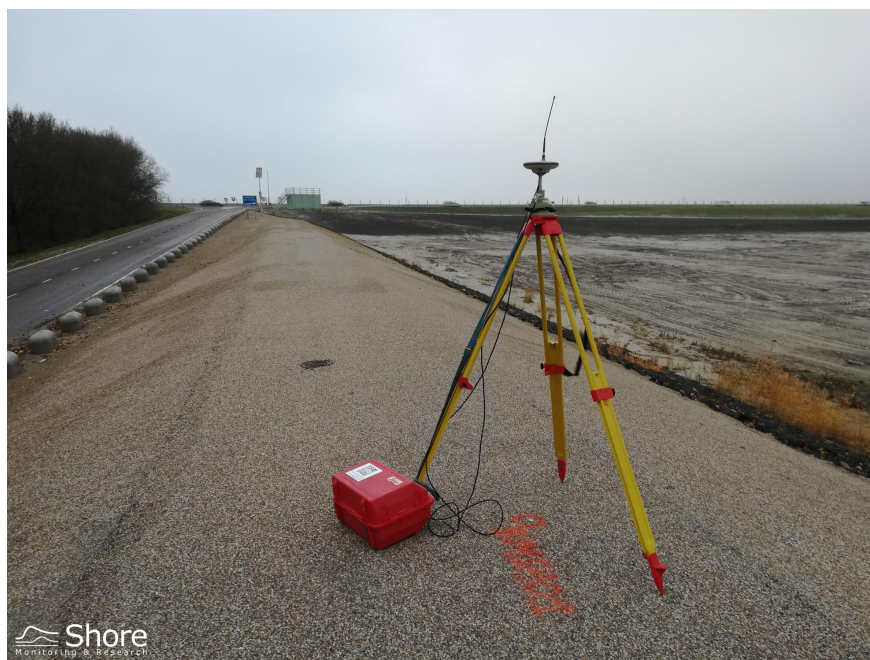
Figure 3.1: GNSS Base station boven BMSH01.
