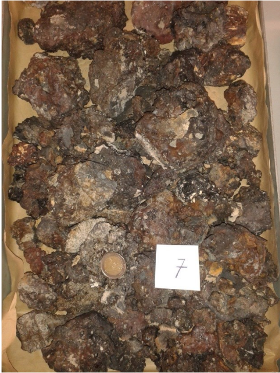
Figure 11: Type 7. This type was most present in the area. There are large and small pieces and there are a lot of different colours: black, white, grey, orange, purple/blue. They are quite heavy and they have a very rough surface.
