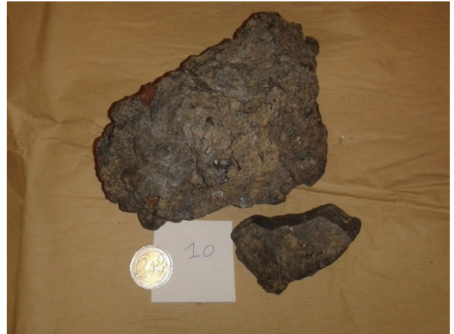
Figure 12: Type 10 is very heavy, especially the large chunk. The small slag is much more smooth than the large one, but the colour is almost the same. Most likely this is steel slag.
