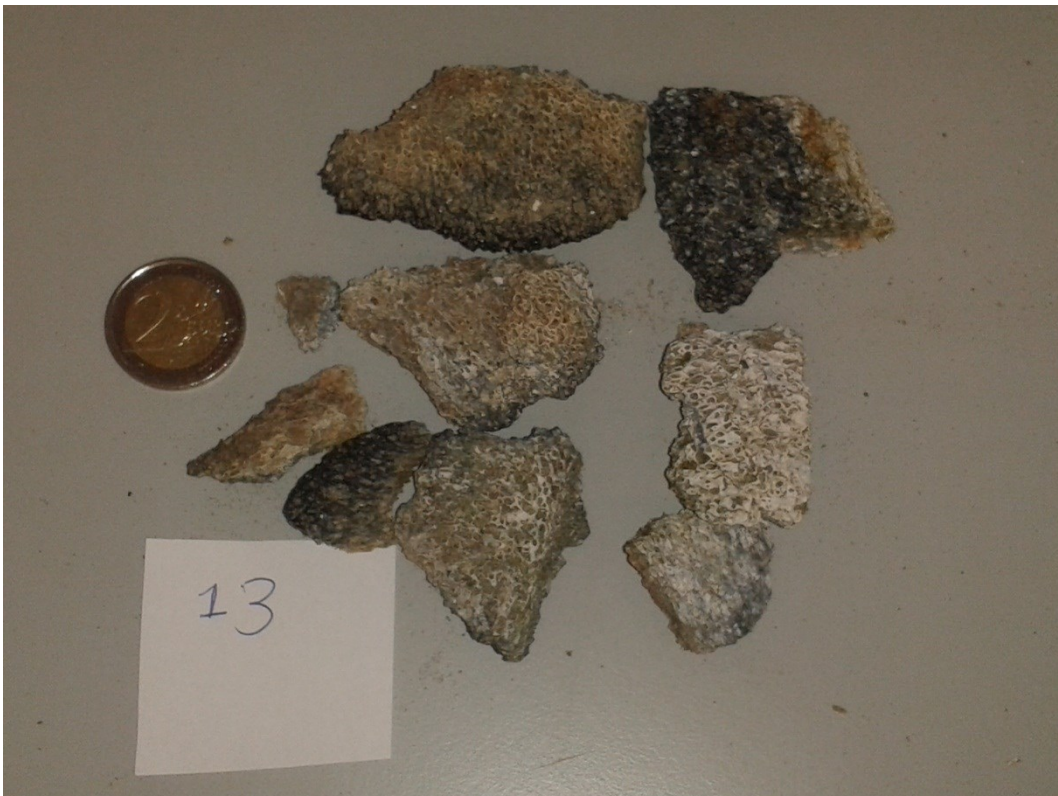
Figure IX: Type 13. Very low mass density, very large pores. It has white and black spots and looks like lime.
