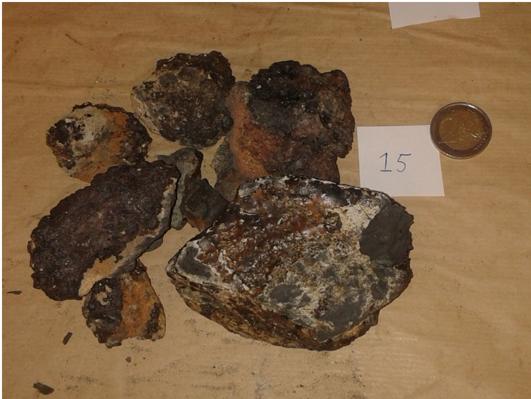
Figure XI: Type 15. These slags have black, grey, brown and orange spots. It looks like they are less layered than type 12. But maybe they are the same type.
