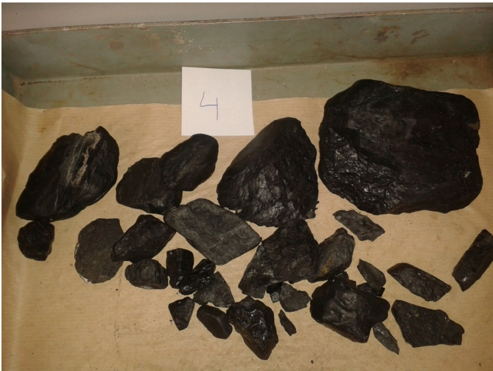
Figure III: Type 4. These slags are very layered, pitch-black and have a very low mass density. They do not peel off. Looks like charcoal and you can draw with it on paper. Possibly this are cokes.
