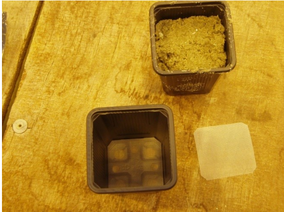
Figure 7: A plastic gauze was put on the bottom of the pots. The pots were filled with sand till 1 cm under the edge.
