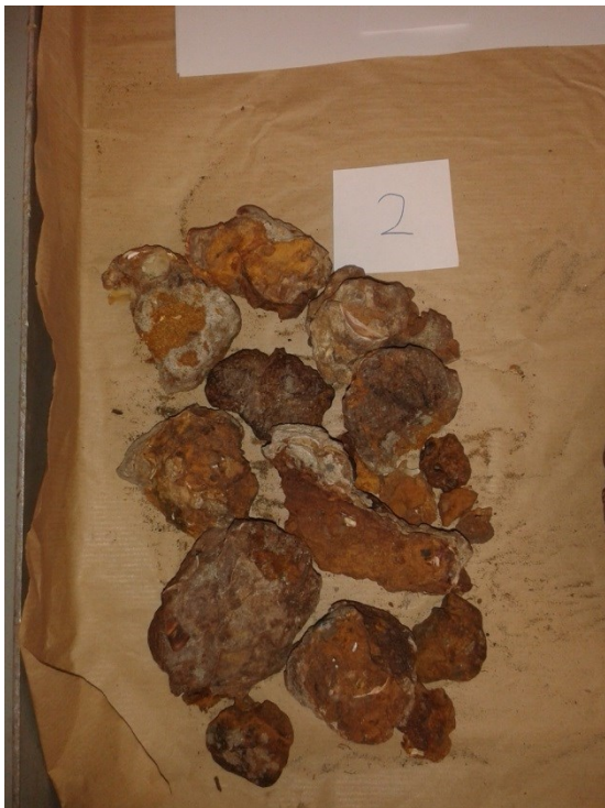
Figure 9: Type 2. These slags have different colours: brown, orange, grey. They all contain a lot of shells. One part contains some rope.
