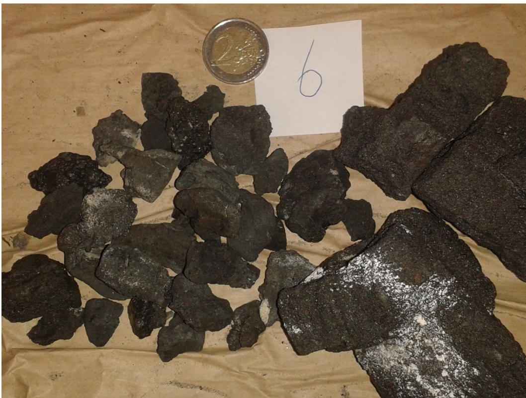
Figure V: Type 6. These slags have a very low mass density, even lower than type 4 and they contain tiny pores.
