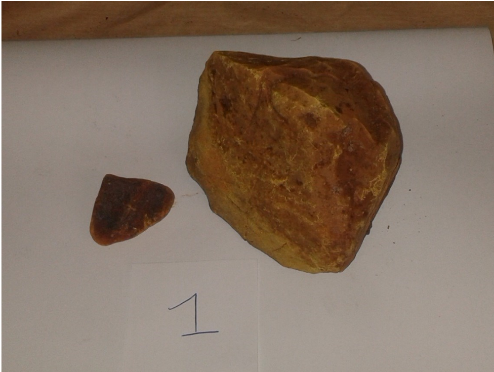
Figure II: Type 1. One side is yellow/brownish (large stone right), the other side is dark brown/orange (small stone left). This slag is not colourfast.
