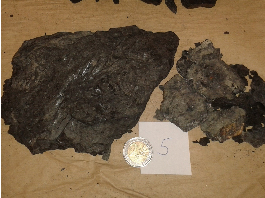
Figure IV: Type 5. These slags are somewhat more grey than type 4 and the mass density is much higher. They are also layered, but they do peel off heavily.
